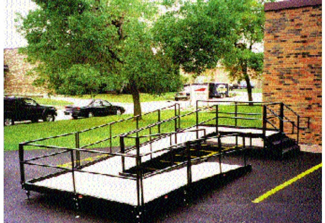
Concrete Deck Ramp System with a 10 and 15 foot ramp, a switch-back platform, a landing and turning platform with stairs and safety gate and double bar handrails.
